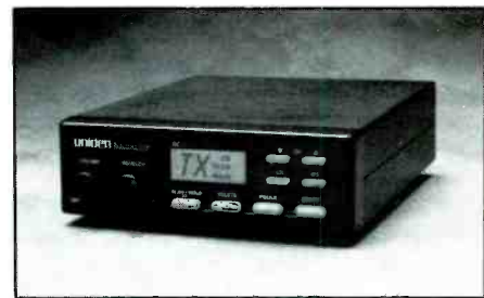
This Uniden BC-1 mobile scanner is factory preprogrammed with state police channels in all states. All the motorist need do is make the state abbreviation show up on the display and the unit does the rest.
