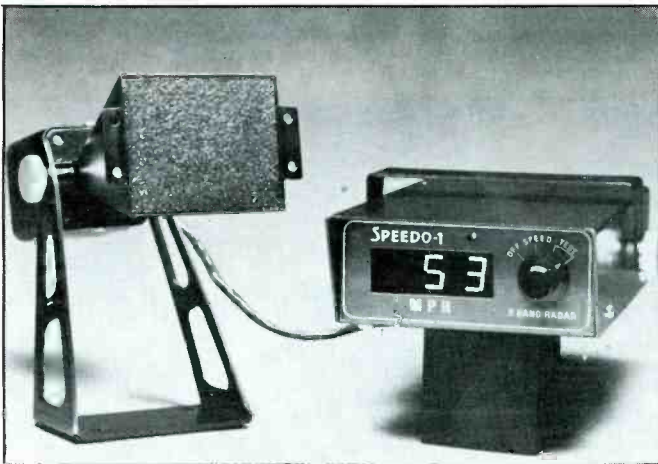
This X-band speed measuring radar unit wasn't made for law enforcement use. It has a few legit uses, but could just as easily be used to mess up police radar.
