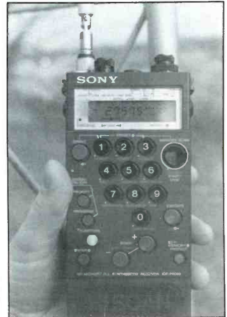
This portable is programmed to monitor 27.575 MHz, which is an active fed channel. Unfortunately, the frequency is often in heavy use by one of the outbander networks.
